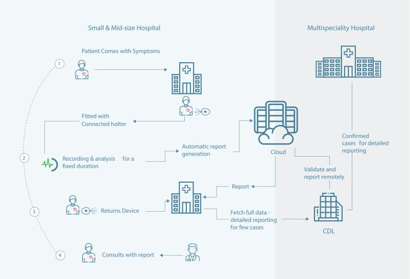
The MIRCaM app running on the connected mobile detects different cardiac conditions and uploads those events to the cloud. These events can be accessed by the physician remotely on his mobile app and reported. In addition to the event reports, a detailed report can be created by the technician either onsite or remotely by analyzing the recorded data on the holter analysis software.
